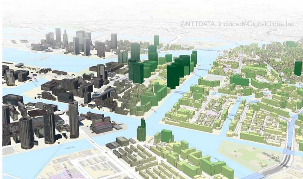
Note: this AW3D model contains more than 11,000 polygons of buildings and rooftop structures. Everything including the textures of building sidewalls was generated solely from satellite data.
