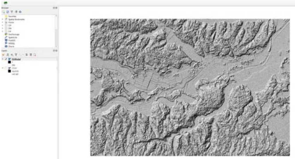
Image: AW3D Enhanced 0.5m DSM data with QGIS 3.10 (after hillshade)
